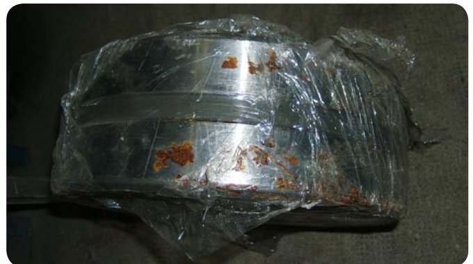
Fig. 3 Bearing, in storage, corroded by humidity.
