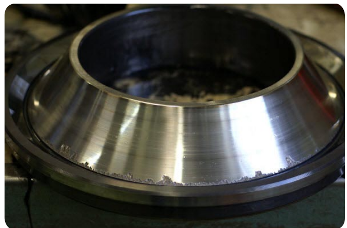
Fig. 2 Bearing made from upgraded steel with spalling
