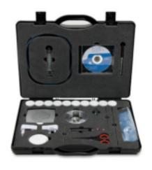
The SKF Grease Test Kit TKGT 1 has been designed to properly apply this methodology. By using it, three different tests can be performed: consistency (patent applied for), oil bleeding properties and contamination. This allows the user to have a good understanding of the grease condition and take decisions directly in the field. The SKF TKGT 1 includes guidelines for properly interpreting the results of the tests.
