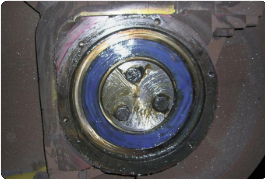
Solid Oil bearing in traveling wheel
