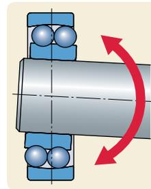
The chart to the left shows the maximum misalignment that can typically be accommodated by various open bearing types. Optimally sized SKF open self-aligning ball bearings can compensate for up to 3 degrees of misalignment, depending on the series. SKF sealed self-aligning ball bearings can accommodate up to 1,5 degrees of misalignment.
